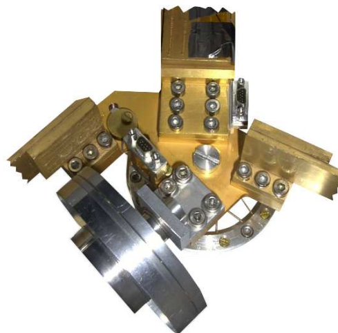
Figure 7: Photograph of the “manifold” in the millikelvin thermal links, showing the Kevlar® wheel support structures. An idea of the scale of this joint can be obtained from the fact that the bolts are M4 size
