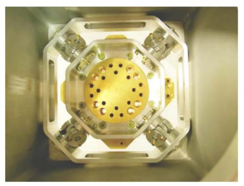
2.5 µW heat leak from 1 K to 100 mK Work stopped when Now copied for use in Clover requirements met
