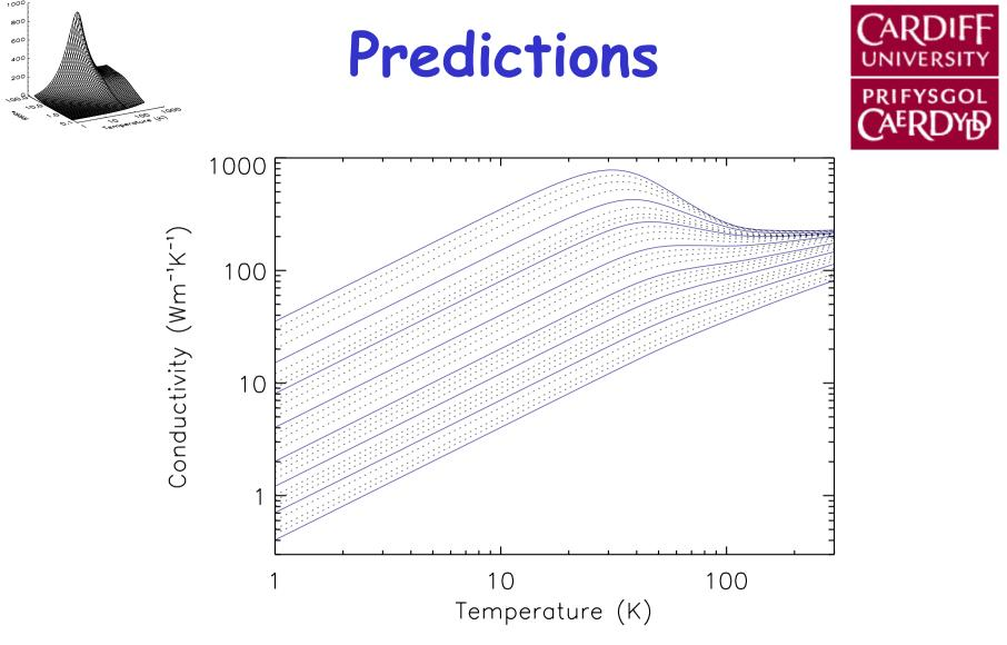
All Al alloys should fall on (or interpolated between) these lines A measurement at any temperature can thus be extrapolated to other temperatures
