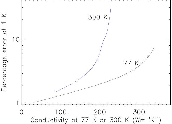
Percentage error in the extrapolated conductivity at 1 K for a 1% error in measured conductivity at 77 K and 300 K
